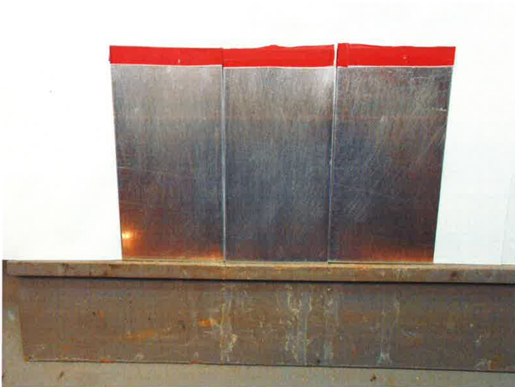
Photo 1: Panels after 1000 hours of QUV testing
