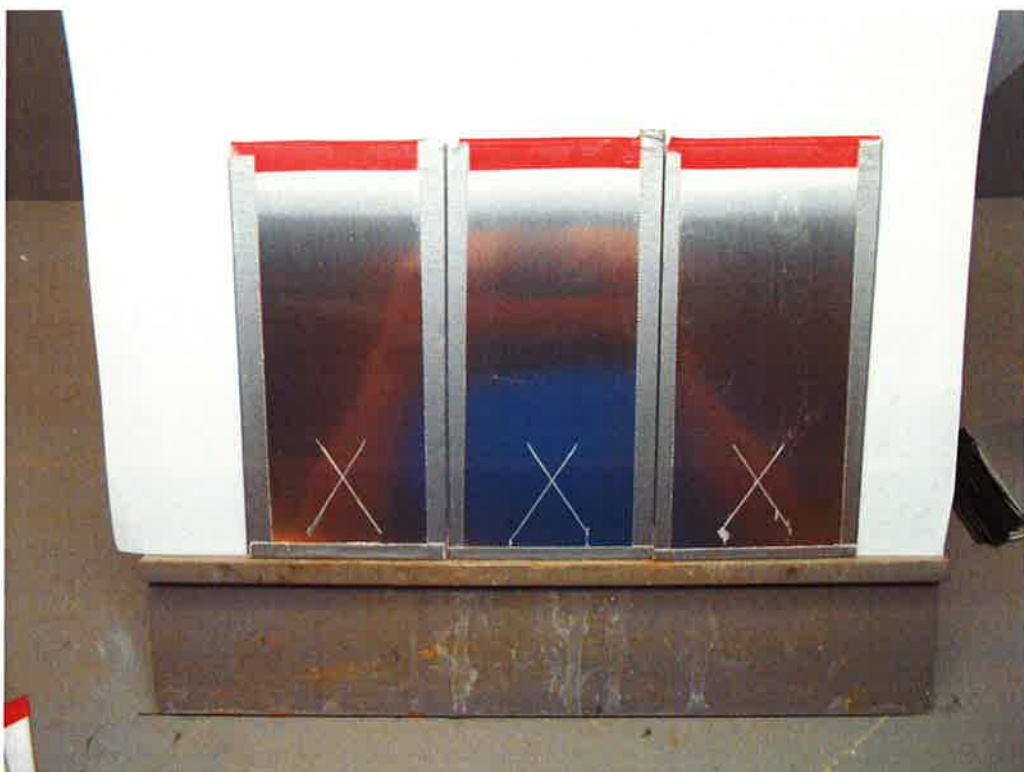
Photo 2: Panels after 1000 hours of neutral salt spray testing
